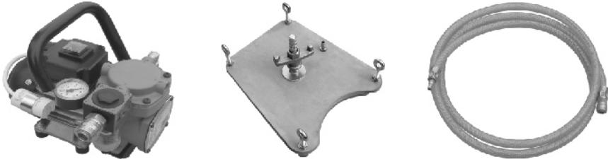
Connect the drill rig with the vacuum plate and the vacuum pump by means of the vacuum tube with the male coupling of the vacuum plate.
